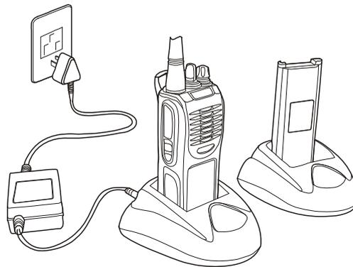
1. Plug the power cable into the adapter.
